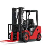
X series Diesel / Gasoline / LPG Capacity 1.5~3.8t
